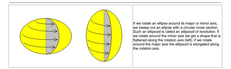
A material with an indicatrix of this shape is called *uniaxial*. There is only one optic axis: down the axis of revolution. Uniaxial materials obviously must have one principal symmetry axis and be tetragonal, hexagonal, or trigonal. Quartz, calcite, corundum, beryl, rutile, tourmaline and nepheline are important uniaxial minerals.
